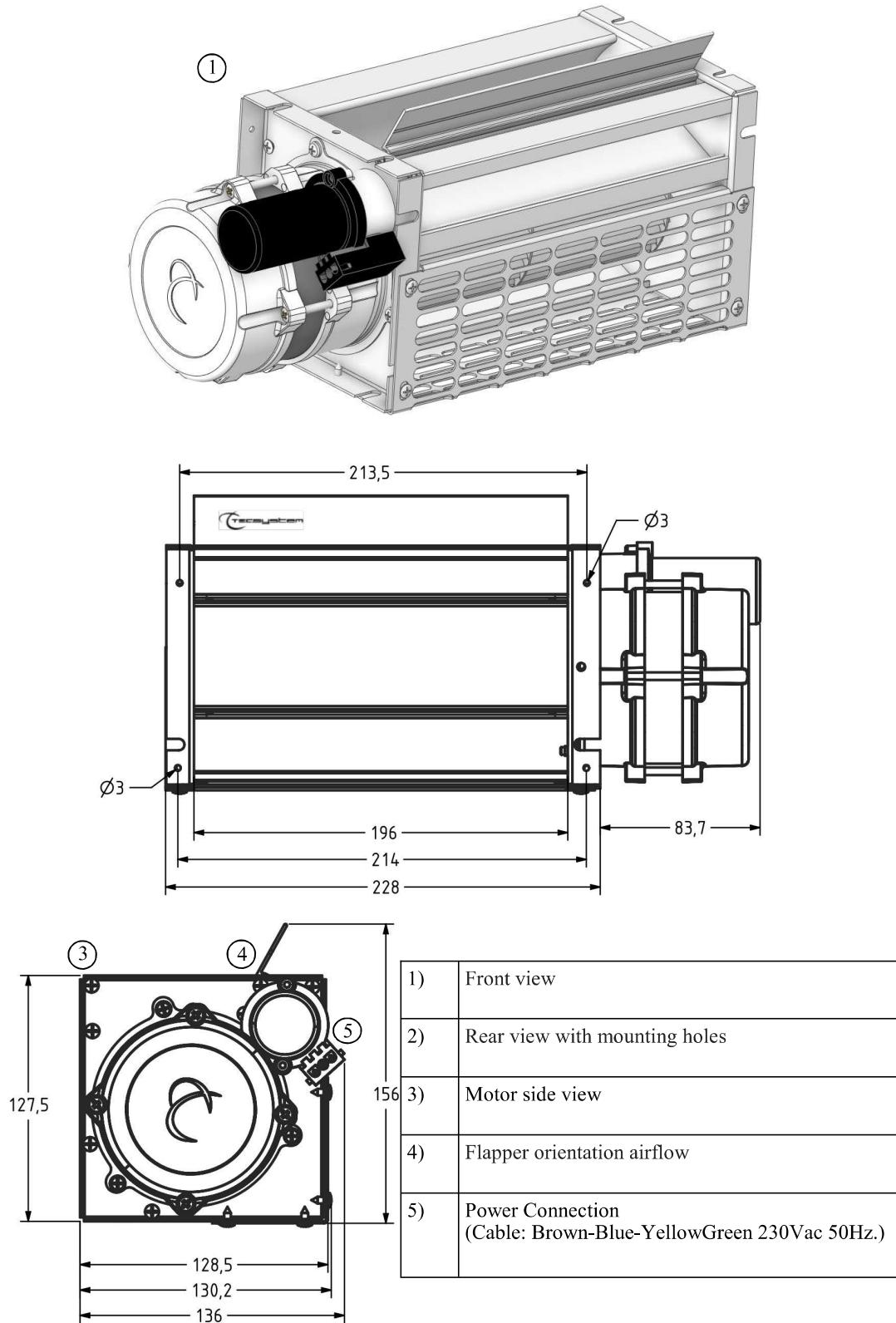
**DIMENSIONS (mm), MOUNTING HOLES AND CONNECTIONS TG360**
